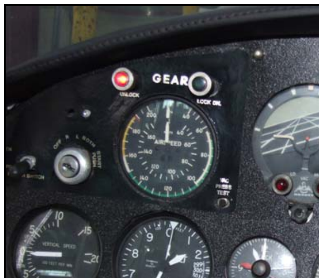
GEAR UP "AMBER/RED LIGHT" FIGURE 32-2
