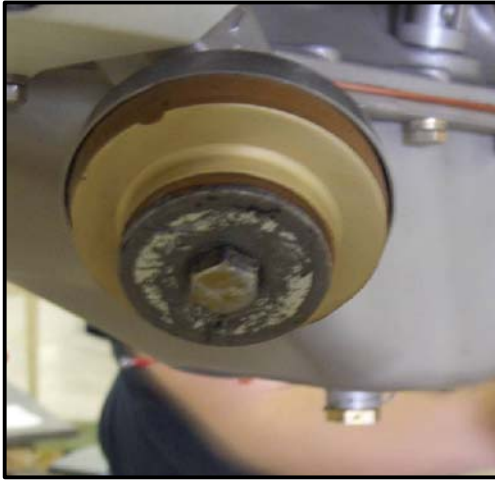
TIGHTEN "DUMMY" BOLTS (NAS6607-15 OR EQUIVALENT) TO COMPRESS RUBBER MOUNTS
