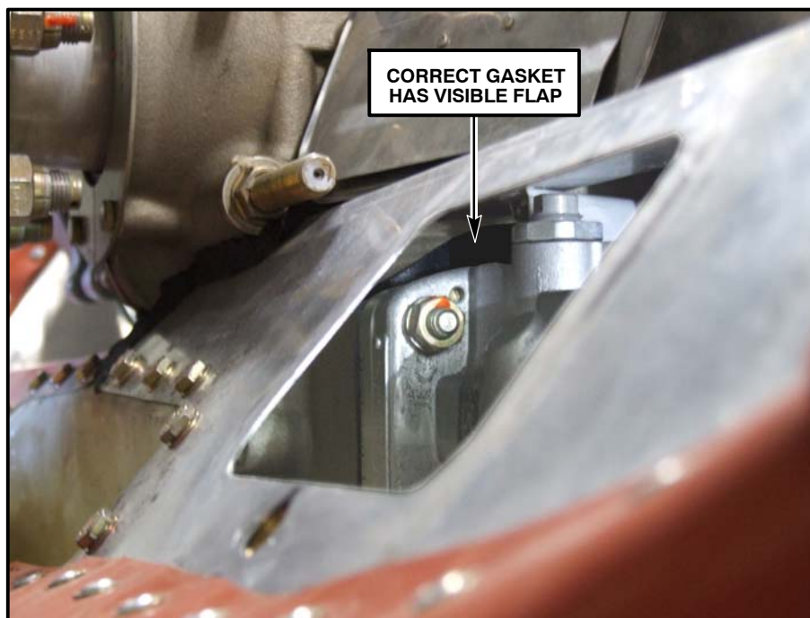
Figure SB M20-323-2 - VERIFY CORRECT GASKET IS INSTALLED THROUGH INSPECTION HOLE
