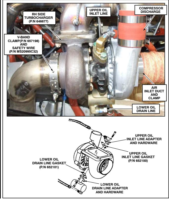
Figure SB M20-299-3 - RH Turbocharger Installed
