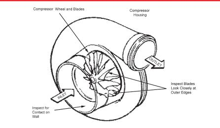
Figure 2 - Turbocharger Inspection Points
