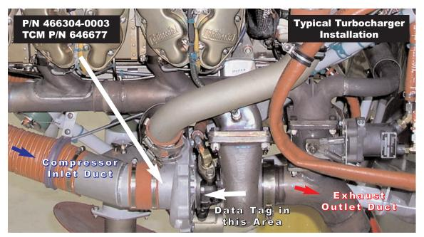
Figure 1 - Turbocharger Installation
