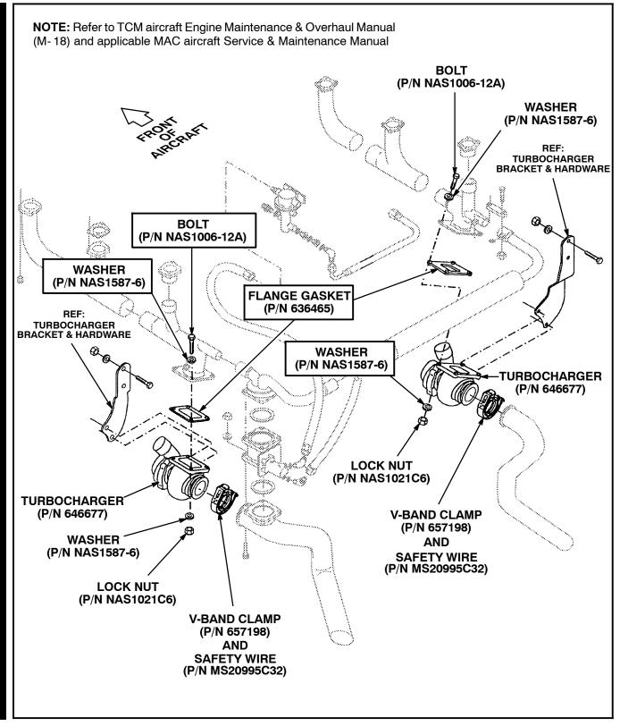
Figure SB M20-299-1 - Turbocharger Hardware and Installation
