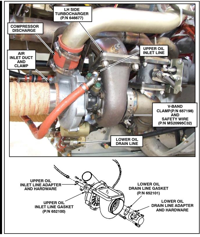
Figure SB M20-299-2 - LH Turbocharger Installed
