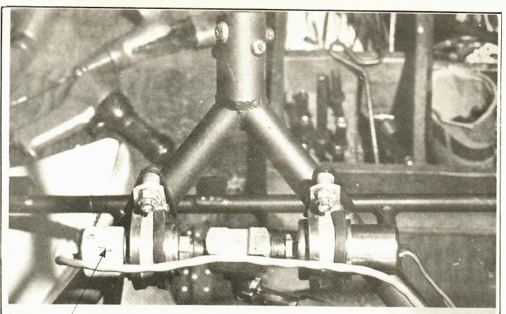
Remove Whitman General vacuum switches, clamps, hose, etc.
