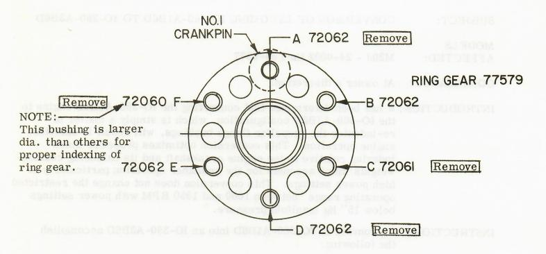
Fig. 1: Propeller Flange Bushing Location For IO-360-A3B6D (Prop moves 60 degrees against rotation)
