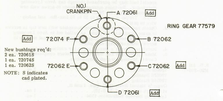
Fig. 2: Tool Needed: ST-115 Install & Remove Prop. Flange Bushing
