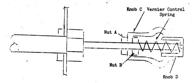
When the control is at either fore or aft limit, the vernier adjustment should not be turned past the point where resistance is felt. When the end of the vernier adjustment travel is reached, knob C should be turned back in the opposite direction approximately at ¼ turn. This will eliminate the possibility of knob D becoming jammed.
