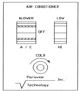
Located on headliner - to identify system switches.
