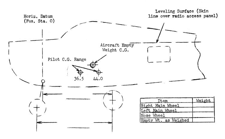
Horizontal Datum is Centerline of Nose Gear Support Bolts (Sta. 0) and is 33.0" forward of Wing L.E. at Wing Sta. 59.25 (Inboard edge of stall strip). MAC is 59.2". L.E. of MAC is 33.1" aft Datum. Leveling means: Edge of skin splice over aft fuselage radio access panel. (Spirit level is used to level.)
